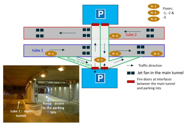
Figure 6 - Example of Courier Tunnel in Annecy (F) including interfaces with parking lots equipped with fire rated doors
