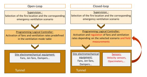
Figure 7 - Illustration of open-loop versus closed-loop control of the ventilation system
