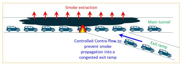
Figure 5 – Example of ventilation strategy in case of fire in a tunnel with a congested exit ramp downstream the fire
