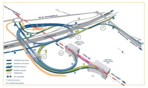
Figure 2 - Example of a complex underground infrastructure -underground interchange between Duplex A 86 and motorway A13 in the Region Ile-de-France. (See monograph 2-8)
