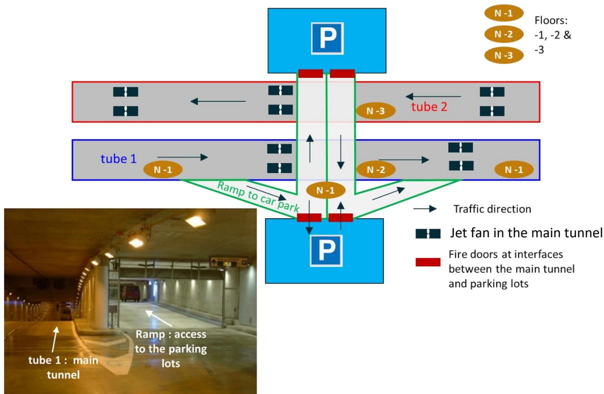
Figure 6 - Example of Courier Tunnel in Annecy (F) including interfaces with parking lots equipped with fire rated doors
