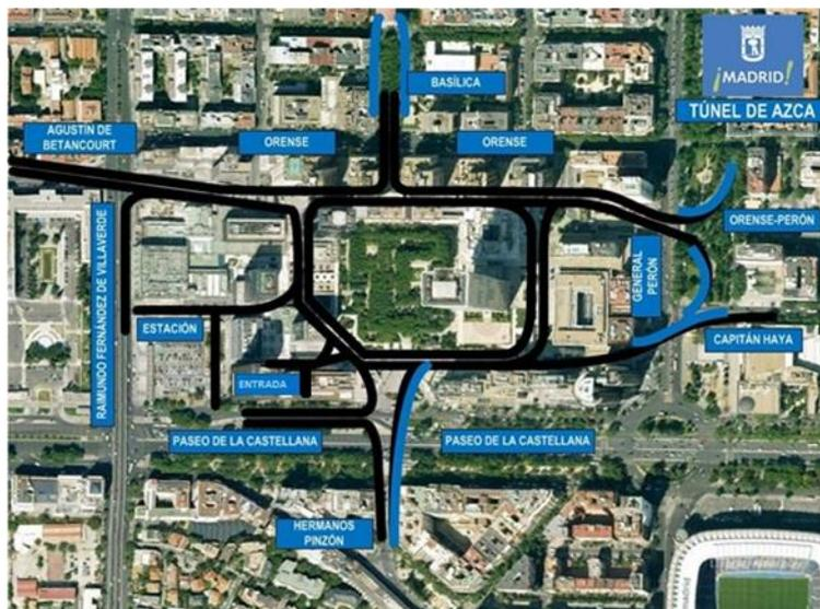
Figure 19 - Layout with the entrance and exit ramps to AZCA Tunnel
