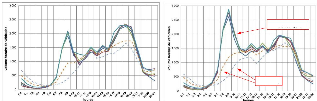
Figure 4 – Daily traffic diagram as «M curve» - traffic directions 1 and 2
